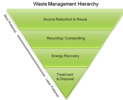
Fig. 3: Graph of a hierarchy ranking the most environmentally sound strategies for the management of non-hazardous municipal solid waste. Source: USEPA, 2013
